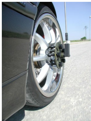
Illustration 23: Aftermarket wheel speed sensor
